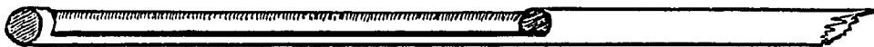
Fig. 1. The trough at the end of the sample introduction device (the "spoon"). The dimensions of the "spoon" are given in the legend to Fig. 2.
